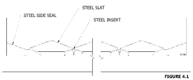
All floor components must be STEEL from wall to wall, including side seals.
